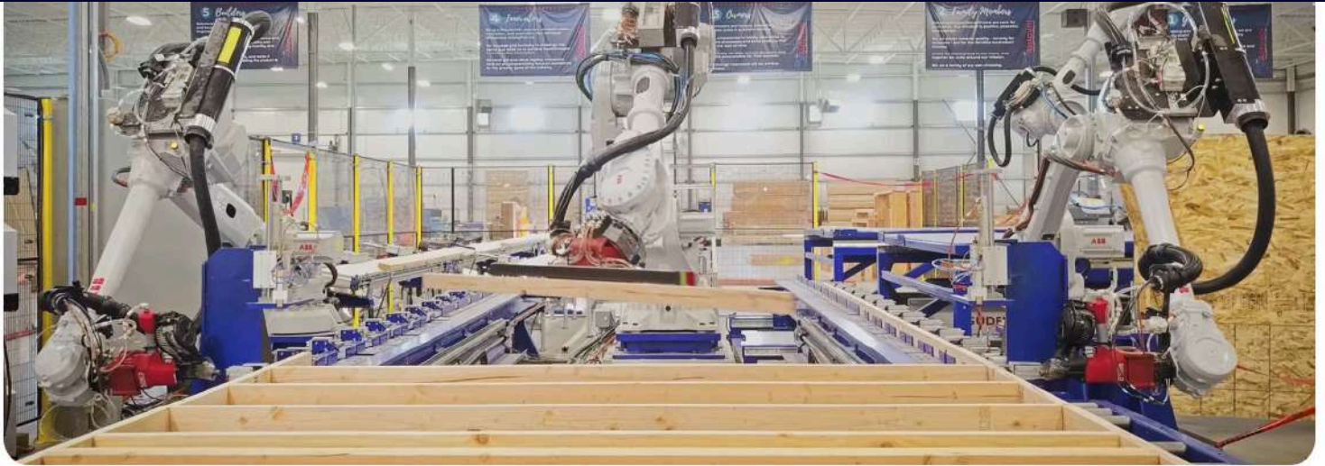
Automated assembly of wooden wall element, by AutoVol
